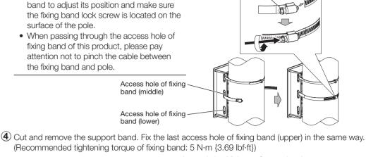
3 Take out one fixing band and pass it through access hole of fixing band (middle), then use a torque
