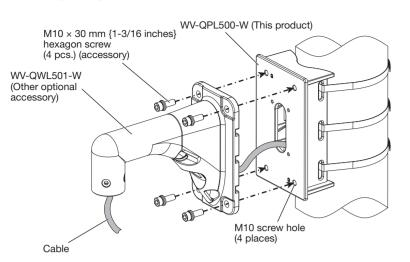
③ As described in the operating instructions of WV-QSR501-W and the camera, install WV-QSR501-W and the camera to the WV-QWL501-W. For the details about the connection of the cable and waterproofing, refer to the operating instructions of the camera.
