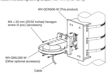
② Connect the cable to the camera and then install the camera. For details about the connection of the cable, the installation of the camera, waterproofing, etc. refer to the operating instructions of WV-QWL500-W and the camera.
