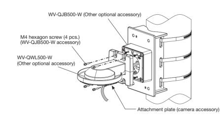
4 Connect the cable to the camera and then install the camera. For details about the connection of the cable, the installation of the camera, waterproofing, etc. refer to the operating instructions of WV-QWL500-W and the camera.
