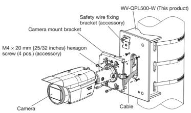
③ Use one M6 x 16 mm {5/8 inches} hexagon screw (accessory) to fix the safety wire of the camera onto the safety wire fixing bracket (accessory). (Recommended tightening torque: 2.45 N·m {1.81 lbf·ft})
