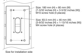
You can attach the camera directly to this product, or attach the camera by using the following bracket combination.
