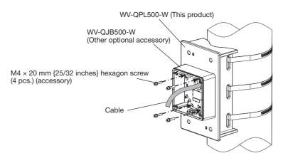
② Install the attachment plate of WV-QJB500-W as described in the operating instructions of WV-QJB500-W.
